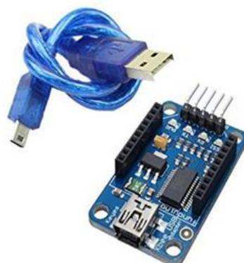
**Fig 3.9** USB ZigBee Adapter
